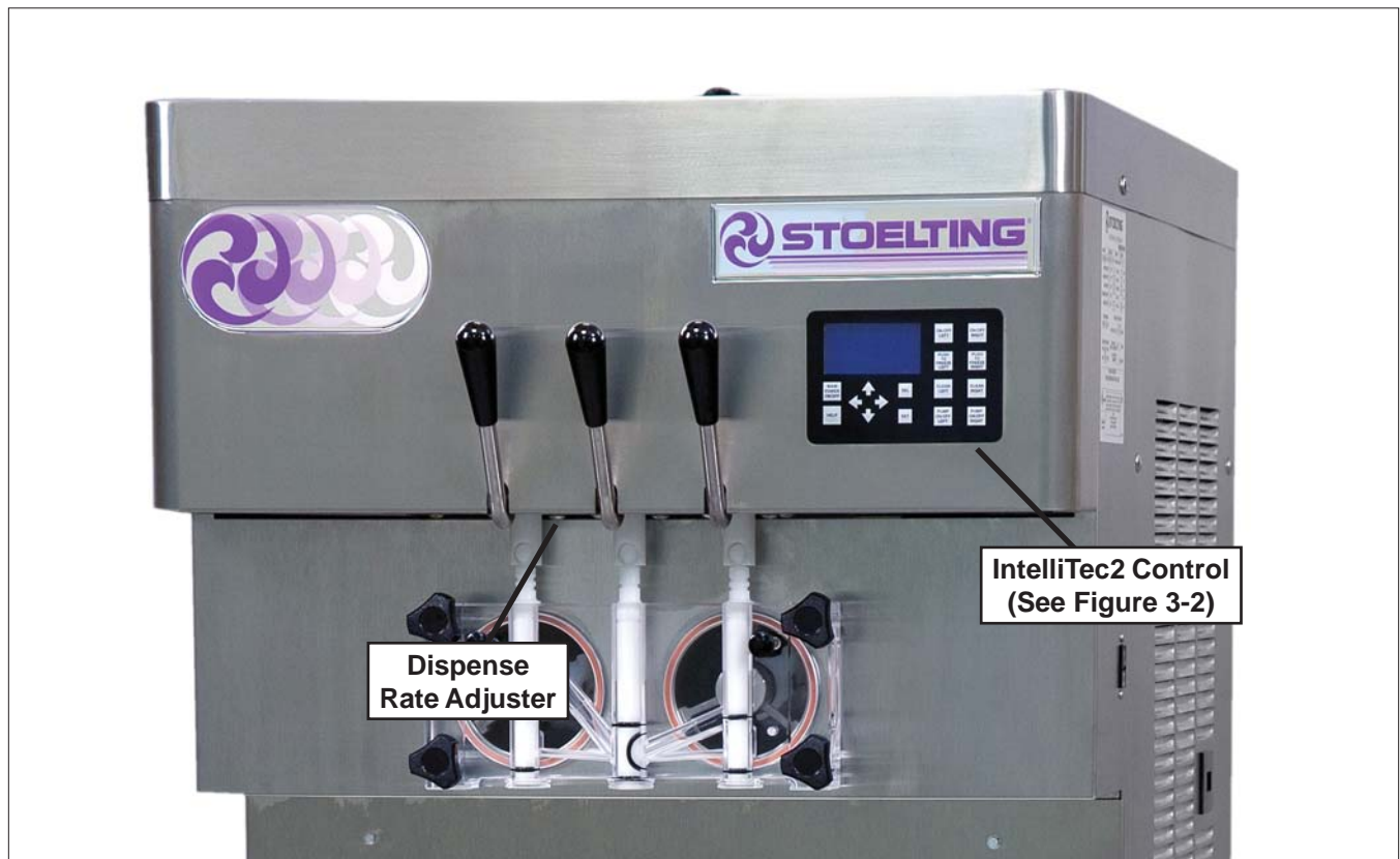
Figure 3-1 U431 I2 Machine Controls
